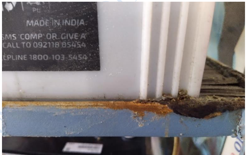
Figure 14 - Galvanic reaction : causes self discharging and degradation.
